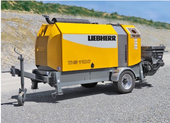
The pump unit is mounted on an extremely rugged steel frame. A sturdy sheet metal housing ensures protection against the weather and noise reduction. A large steel grid provides protection for the cooling system in the suction area and guarantees reserves for cooling performance. All components are compactly integrated and encased in a state-of-the-art design.
